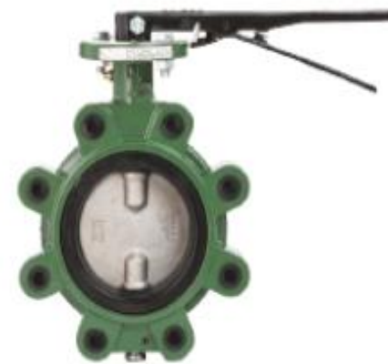
Lug Type Ductil Iron Body Buna Seat Zinc Plated Ductil Iron Disc Sizes: 2" - 36"
