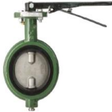
Wafer Type Ductil Iron Body Buna Seat Zinc Plated Ductil Iron Disc Sizes: 2" - 36"
