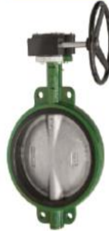
Wafer Type Ductil Iron Body Buna Seat Stainless Steel CF8M Disc Sizes: 1" - 36"
